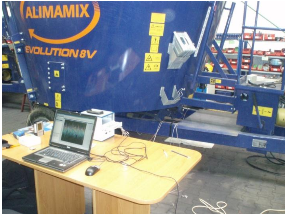
Fig. 5. Conditions for performance of strain gauge measurements
