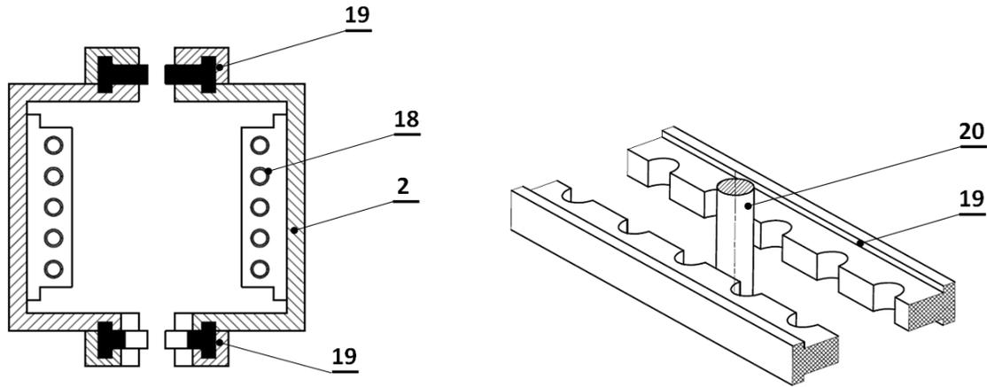
Fig. 4. Arrangement of electrodes and sealing of the chamber and spindles
