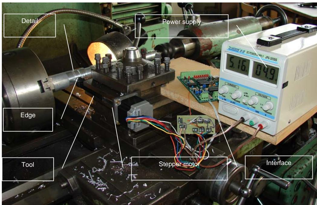
Fig. 8. Turning using controlled PC mechatronics tool
