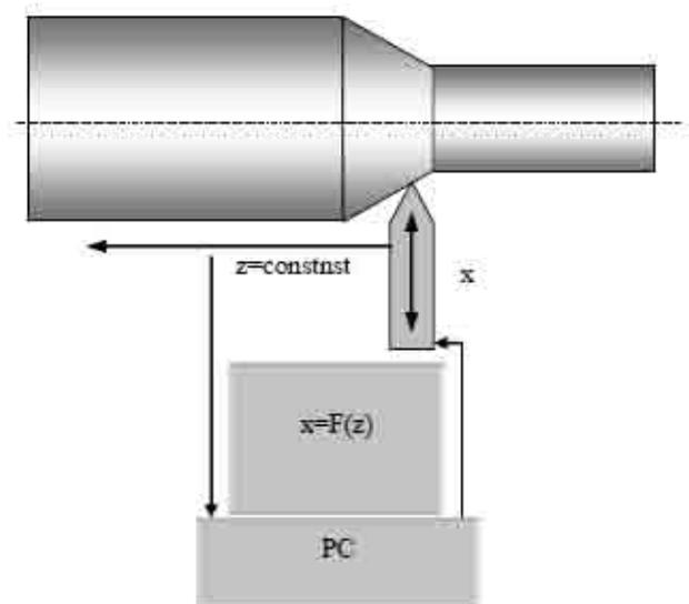
Fig. 2. Idea of mechatronics PC controlled turning tool
