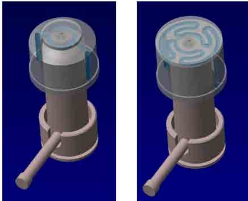
Fig. 4. Cooling bushes with conformal channels manufactured by laser incremental techniques [6]
