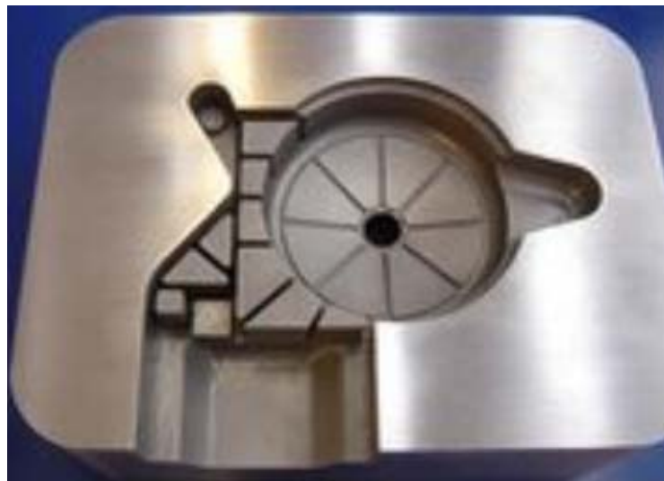
Fig.3 Front of the cavity insert in which the honeycomb shaped cooling was made [3]
