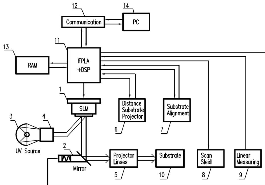
*Fig.2 System for direct transfer of the image by sub-pixel scrolling method
