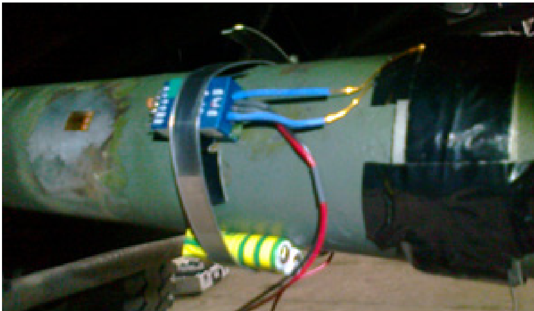
Fig. 7. Measurement system while being mounted on the drive shaft [own research]
